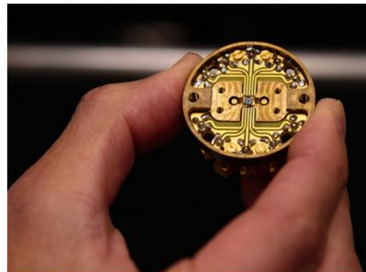
NTT's silicon single-electron device chip mounted on a sample holder for NPL's high-precision current measurement system
